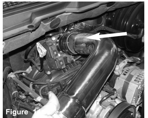
Figure 11 With provided M8 vibra mount install to the threaded fitting located on the fender frame next to air box bracket.
