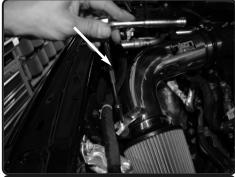
17. Tighten and secure the vibramount using 10mm socket or wrench.
