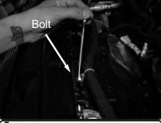
**5.** Locate the bolt on fender frame, loosen using 13mm wrench or socket. Save bolt for later install.
