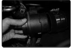
**10.** Install the MAF sensor to the hose. Make sure the arrow is going in the direction towards the turbo.
