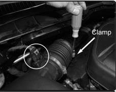
**2.** Loosen the clamp on the turbo housing. Disconnect MAF sensor.
