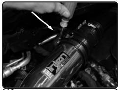
**16.** Position for best fit and tighten the clamp on step hose using 8mm nut driver.
