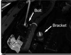
7. Now install the bracket, secure using bolt from previous step. This will be support bracket for the intake tube.
