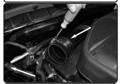
**8.** Now install the 3-1/8" straight hose with clamps to the turbo housing. Tighten clamp on turbo housing.
