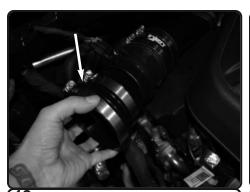
**12.** Install the step hose to the MAF sensor with clamps provided, tighten the clamp on MAF sensor.
