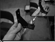
**6.** Now attach the vibramount to the thredded part of the bracket. Secure and tighten.
