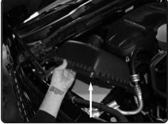
7. Carefully un-clip upper half of airbox and remove.
