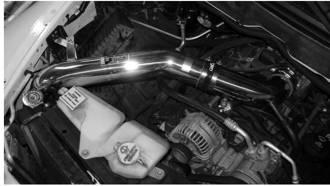
Congratulations! You have just completed the installation of the World's first tuned intake system, the Power-Flow intake, featuring MR Technology. Periodically, check the system for fitment, this will enhance the life of your Power-Flow system, failure to do so will void the warranty.
