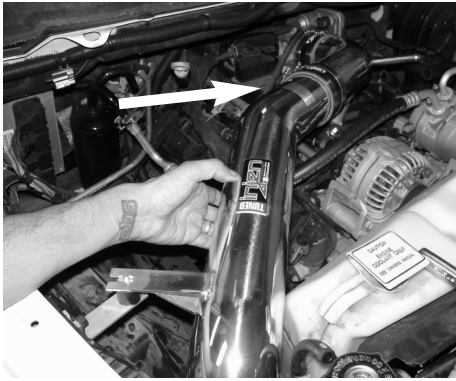
Position the lower intake assembly to the upper intake assembly.
