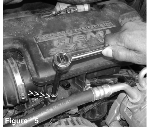
Figure 5 Loosen and remove the two front bolts that secures the intake resonator to the intake manifold.
