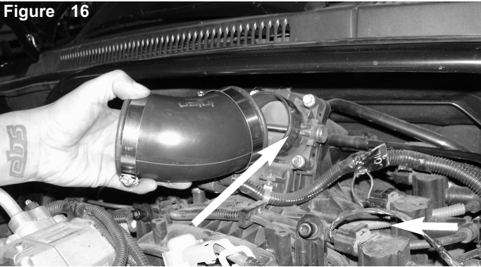
Install the 2-3/4" side of elbow hose with clamps provided to the throttle body.
