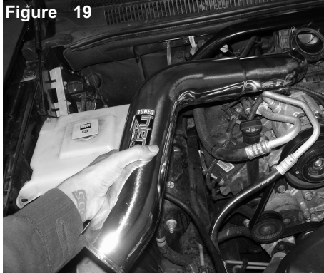
Position the intake tube to the elbow hose and bracket to the vibra mount.
