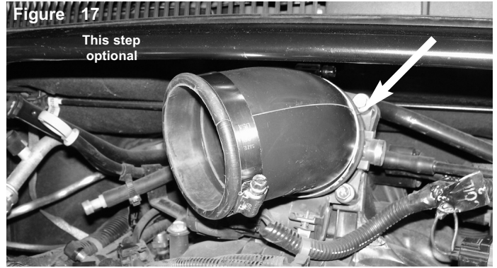
Position the hose so that it does not hit the support brace.
