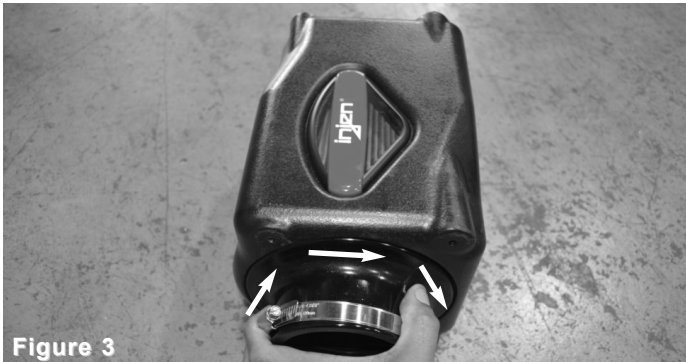
Figure 3 Once the filter is seated correctly and flat, rotate the filter 1/4" turn in either direction left or right and secure. Filter has built in lock.
