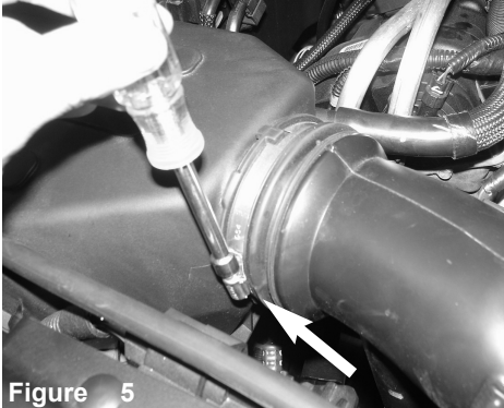
Figure 5 Loosen the clamp on the air box using 8mm nut driver.
