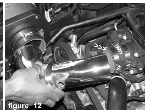
figure 12 The air intake is now lowered into the engine compartment, the upper end is pressed into hose on the throttle body.
