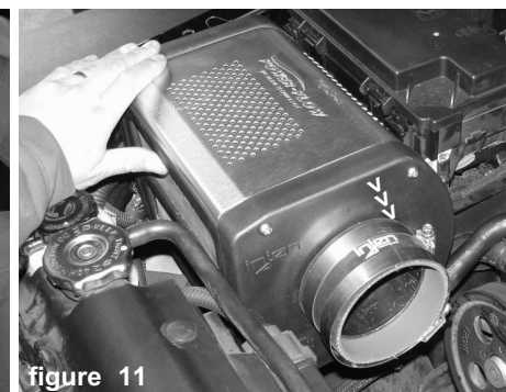
figure 11 The three metal pegs are aligned and pressed into the stock grommets. The 3 3/4" straight hose is pressed over the the velocity stack. Two power bands are used on the hose. The clamp on the velocity stack is now tightened.
