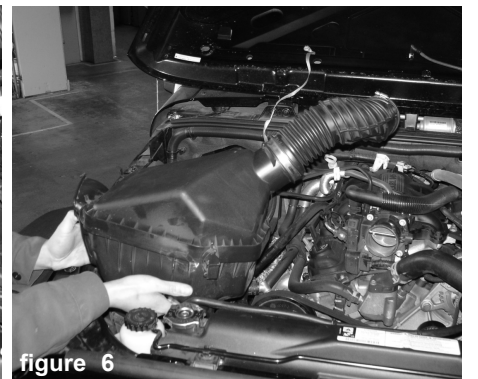
figure 3 Unplug the crank case breather hose from the air box vacuum port.
