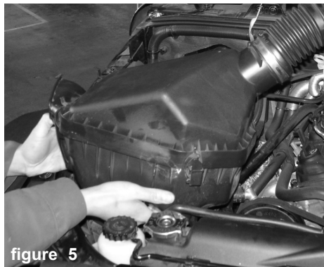
figure 2 Loosen the metal clamp that secures the air duct to the throttle body.
