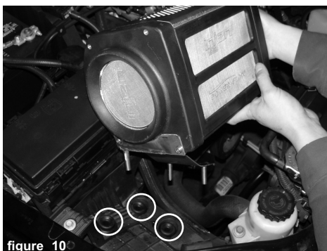
figure 10 Once the bracket has been installed, continue to lower the entire power box in the the engine compartment. The three metal pegs are aligned to the stock grommets and plugged into the grommets. Page 2 of Part# PF5002
