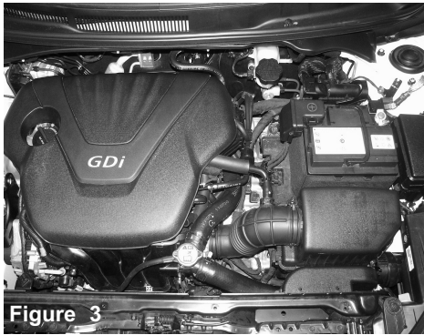
Figure 4 Carefully lift up and remove the engine cover.
