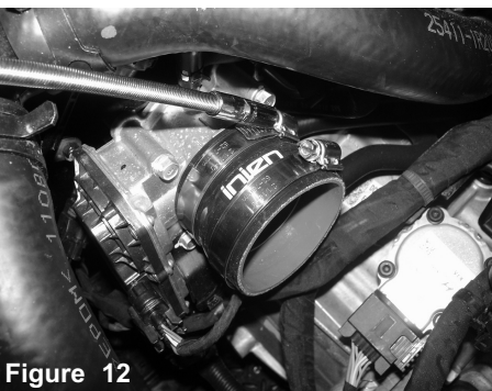
Figure 9 Pull back the intake tube from the throttle body.
