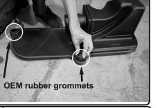
holes on air box. These will be used to secure the injen evolution air box.
