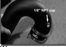
**14.** If vehicle is not equipped with vacuum line, remove the 1/8" brass fitting and install the provided 1/8" NPT cap. Secure and tighten.
