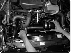
**18.** Position tube to sit in the center, and tighten the clamp.
