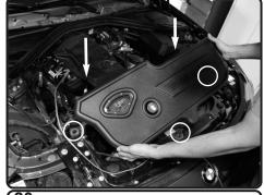
**20.** Install the air box assembly into the vehicle. Position the mounting points to the OEM location and secure.
