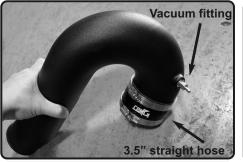
**13.** Please verify if vehicle is equipped with vacuum line, this fitting will be used. Install the provided 3-1/2" straight hose with clamps provided to tube.
