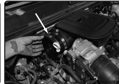
**11.** Place the 4.25"-4.50" step hose and two #72 clamps onto the turbo inlet. Tighten the clamp on the turbo inlet side for now.
