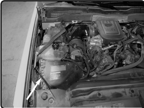
**1.** Stock intake system shown. Remove support brace.
