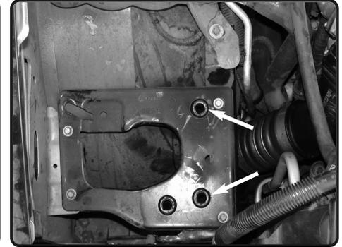
**9.** The factory air box assembly bracket is shown in the photo. Arrows indicate the grommets where the Injen air box mounts will go.
