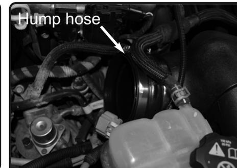
**12.** Place the 5.00" hump hose and two #80 clamps onto the Injen intake plenum on the injen air box.
