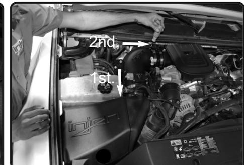
**13.** First slide the big end of the intake pipe into the 5.0" hump hose on the air box plenum. Then slip the smaller end into the 4.25"-4.50" step hose on the turbo inlet. Once intake is adjusted, tighten all clamps.
