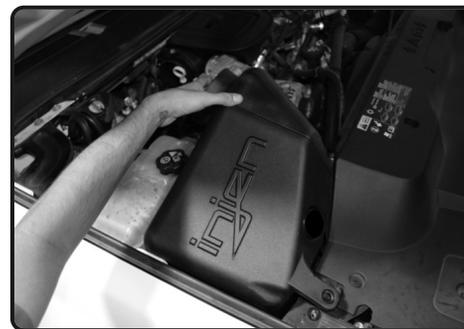
**10.** Lower the Injen air box into the engine bay. Make sure the pegs under the Injen air box goes into the factory air box grommets on the air box tray from figure 10
