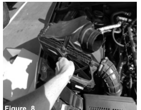
Figure 8 Lift up and pull up the factory air box and remove out of vehicle.
