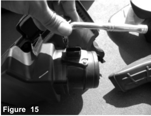
Figure 16 Carefully remove the MAF sensor.
