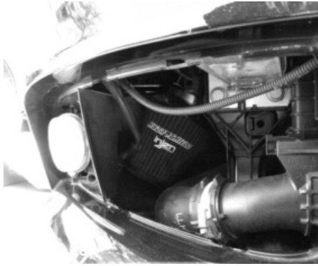
Install the air filter to the tube and tighten using 8mm nut driver.
