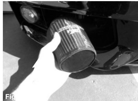
Figure 18 Install the step hose to the turbo and tighten the clamp on turbo only
