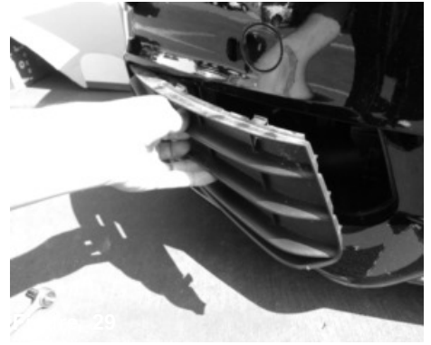
Re-install the front valence.
