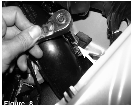
Figure 8 With 10mm socket and extension, loosen the bolt holding in the plastic snorkel assembly.
