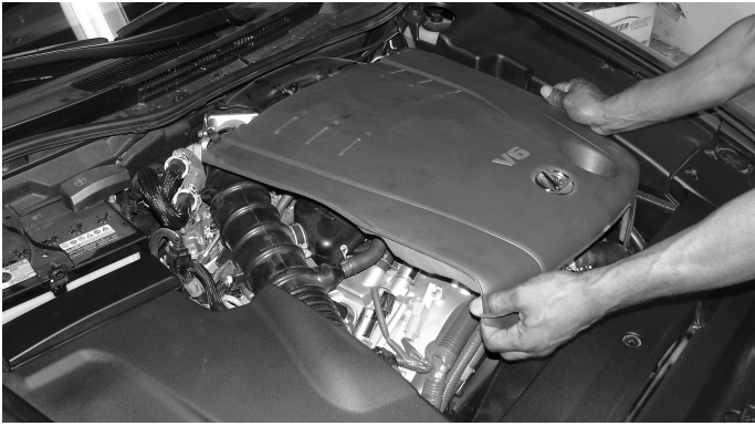
Pull the engine cover from the intake manifold by firmly pulling in a upward motion.
