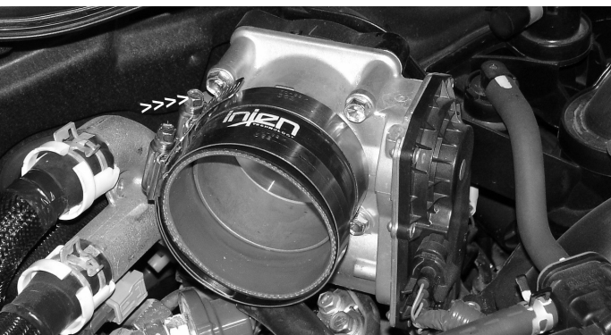
Press the 3 straight hose over the throttle body and use two power clamps. Use two power-clamps and be sure to tighten the clamp directly over the throttle body end for now.
