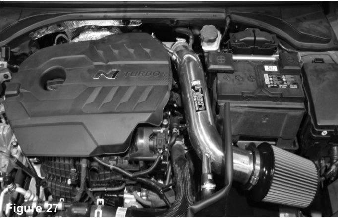
Figure 27 Congratulations! You have just completed the installation of the World's first tuned intake system. Periodically, check the system for fitment, this will enhance the life of your Injen SP system, failure to do so will void the warranty.
