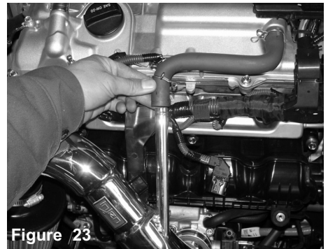
Figure 23 Place the factory breather line to the long 5/8 nipple welded to the pipe.
