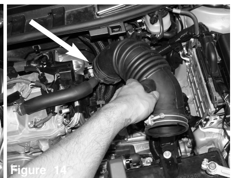
Figure 11 Pull back the ECU harness that is attached to the back of the bottom half of air box.
