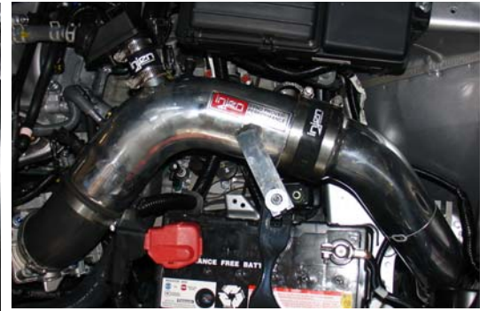
Congratulations! The installation is now complete. align the entire intake for best possible fit, then continue to tighten all nuts, bolts and clamps. Periodically, check the alignment of the intake to prevent damage to the intake system.
