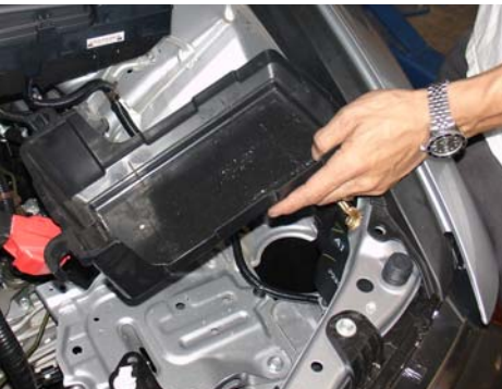
Once the battery has been removed, continue to remove the battery tray from the metal frame.
