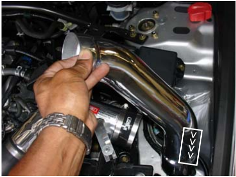
The secondary intake is now inserted into the resonator opening as shown above.
