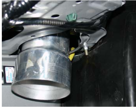
The 3 1/2" inlet on the secondary intake will sit just below the resonator opening as shown above.
