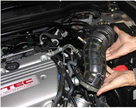
Loosen clamps and remove the air intake duct as shown above.
