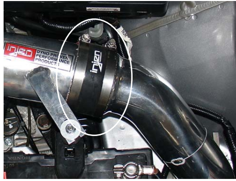
The secondary intake is pressed into the 3 1/2" hose located on the end of the primary intake.
