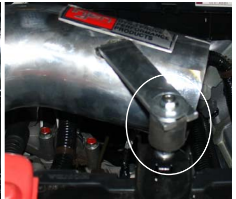
The intake bracket is now aligned to the vibra-mount stud. Use the m6 flange nut and fender washer to secure the intake in place.
