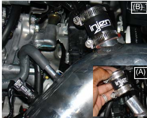
Take the 2" long CCV hose, place one clamp on each end of the hose. Press the CCV hose over the large intake port as shown above (A). The CCV hose is in installed and clamp is tightened (B).
