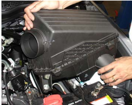
Loosen bolts and take out entire air intake box.
