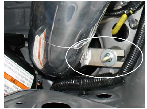
Once the top end of the secondary intake has been inserted into the primary hose, continue to align the intake bracket to the vibra-mount stud. Use the m6 flange nut and fender washer to secure the intake.
