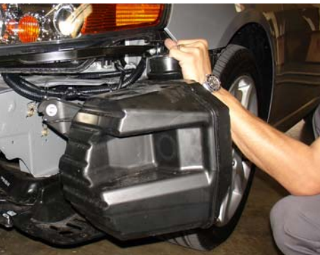
Note: In order to proceed to the next step, removal of the front bumper will be required. Loosen bolts and remove the air resonator box.
