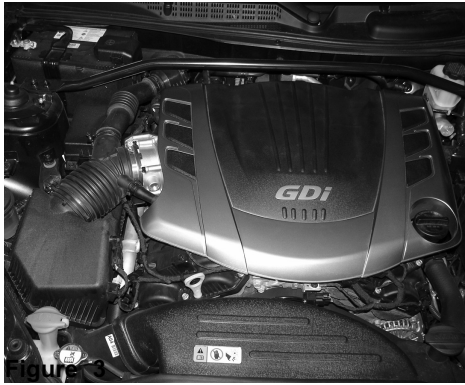
Figure 3 Stock air intake cleaner and air ducts shown in this picture. Before getting started with the installation, disconnect the negative battery terminal.
