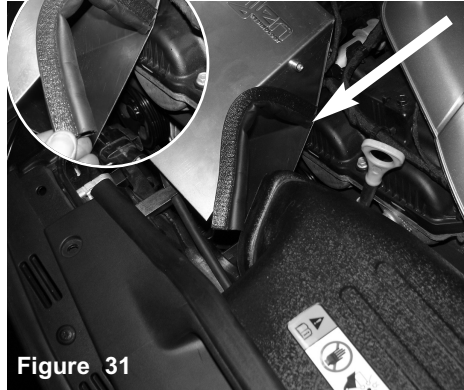
Figure 31 Attach the provided rubber trim to the heat shield like image above. Install the factory ram scoop and position for the plastic to sit inside of the new injen heat shield.
