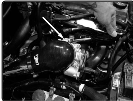
**17.** Now position the intake tube for best fit, close hood to see the cobrahead is in the correct position and does not hit. Tighten both clamps using 8mm nut driver.
