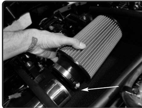
**18.** Install the filter to the intake tube.
