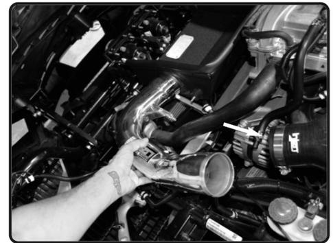
**15.** Now install intake tube and position the tube through heat shield and bracket to vibramount on heat shield. Install to cobra head, Do not tighten.
