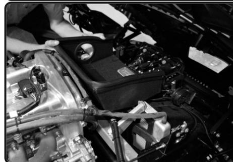
10. Install the heatshield and position the brackets to the vibramounts.
