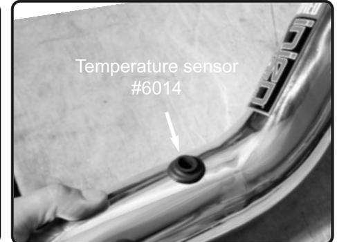
7. Install the temperature sensor grommet to the hole on intake tube.
