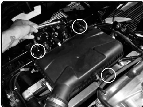
4. With 10mm socket and extension and ratchet, loosen the 3 bolts holding in the air box.
