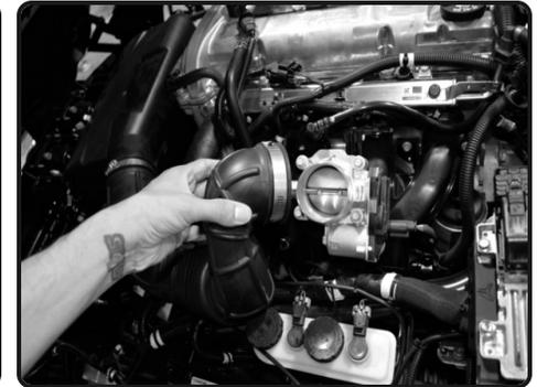
3. Now lift up and pull back the intake tube from the throttle body.
