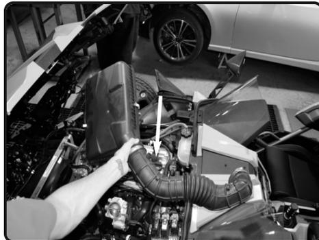
5. Carefully lift up and remove the entire stock air box assembly.
