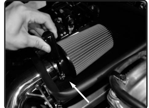
**19.** Tighten filter using 8mm nut driver.
