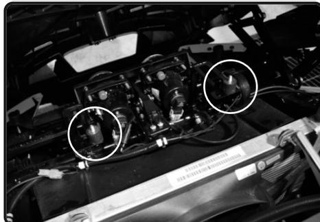
9. Secure and tighten the vibramounts.
