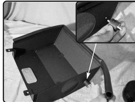
6. Install the provided rubber trim to the top of the heat shield. Notch corners for easy installation with pliers. Install the m6 vibramount to the threaded insert on heat shield.
