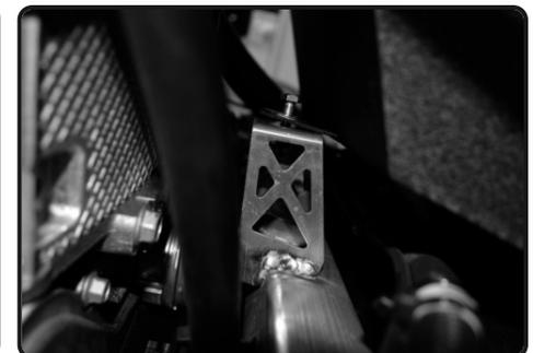
11. Now secure the back bracket to the factory air box mounting position. Secure using provided m6 hex screw and fender washer.
