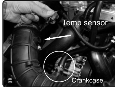
7. Carefully pull out the temperature sensor out of intake tube. With pliers, disconnect clamp on crankcase line and pull hose away from the fitting. .
