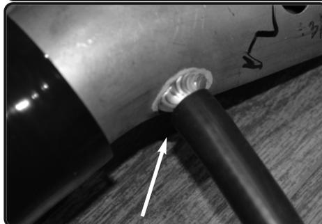
**22.** Attach the crankcase hose to the 1/2" fitting on tube. Secure using original clamp.
