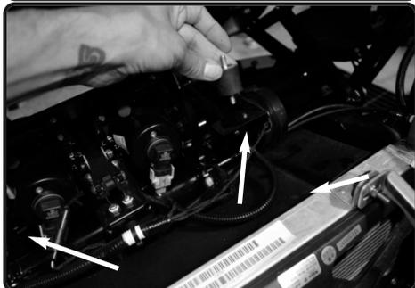
8. Now install the vibramounts to the 2 factory mounting position of the air box.
