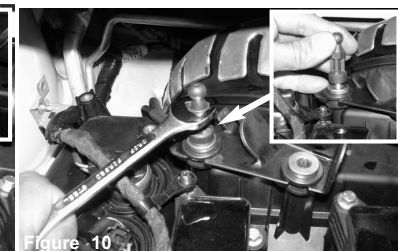
Figure 10 Now loosen the engine cover fitting using 12mm wrench. Remove and save fitting and grommet with spacer for later install.
