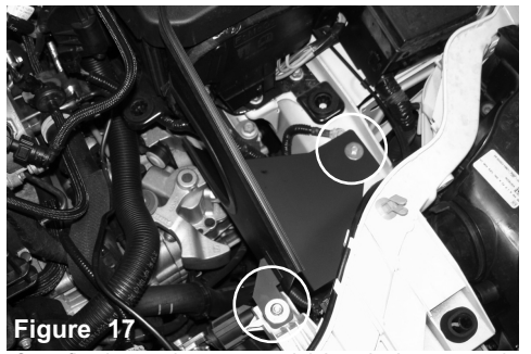
Figure 12 Install the vibramount to the thredded insert from step 5. Secure and tighten.
