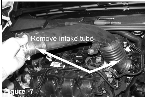
Figure 7 Carefully lift up and remove the stock intake tube from the vehicle.
