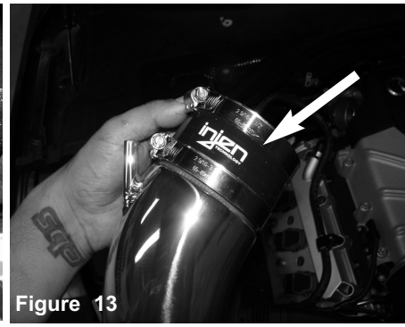
Figure 13 Attach the 3" hose with clamps provided to the intake tube. Do not tighten.
