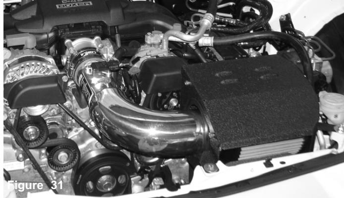
Figure 30 With provided M6 button head screws, secure the cover and tighten. Re-position if necessary. NOW CONNECT BATTERY TERMINALS. START VEHICLE AND LET IDLE FOR 5 MINUTES.
