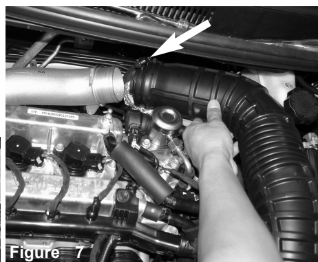
Figure 7 Use a 10mm socket and ratchet and loosen the 10mm clamp bolt on the air duct located on the Turbo charger compressor outlet. Pull the air duct from the outlet.
