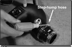
**12.** Attach the step hose with clamps provided to the intake tube. Tighten clamp on tube only using 8mm nut driver.
