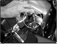
**4.** Now disconnect the Crank case fitting from the intake tube and pull back from tube.
