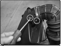
**6.** With T25 torx bit, loosen the 2 screws holding in the MAF sensor.
