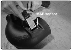
10. Install the MAF sensor into the tube.
