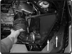
**5.** Now Lift up air box from vehicle and remove complete stock air box assembly.
