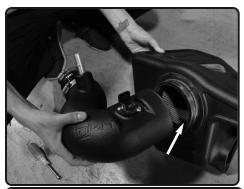
**13.** Install the intake tube assembly to the filter. *Do not tighten.*
