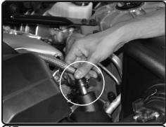
**17.** Re-connect the crank case line to the fitting on the intake tube. Make sure you hear the click to make sure its secured.
