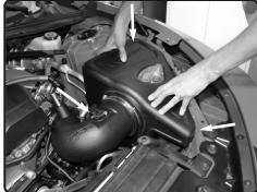
**15.** Make sure the intake tube is secured on the turbo. Make sure the airbox is seated properly. Position for best fit.
