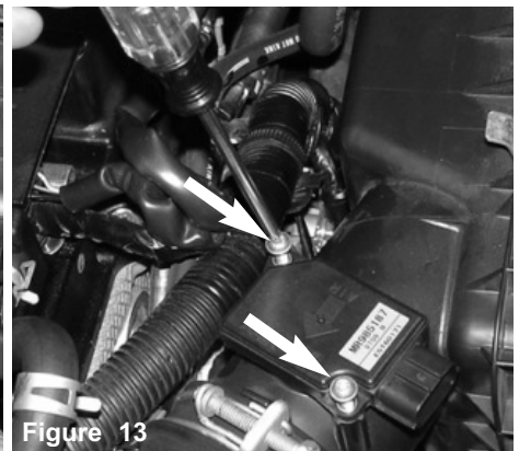
Figure 13 An allen screwdriver is used to loosen the two stock screws from the mass air flow sensor.
