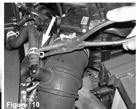
Figure 10 The tension clamp is compressed and pulled from the crank case vacuum hose located over the air intake duct.
