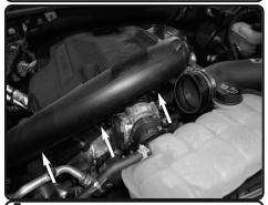
**5.** Push aside the OEM turbo inlet pipe out of way allowing for clearance.
