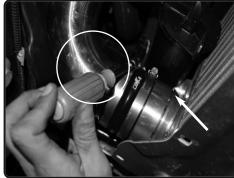
**24.** Attach the bottom part of the charge pipe and tighten using 8mm nut driver. Re-connect the diverter valve hardline. Re-install coolant reservoir and re-connect intake system.
