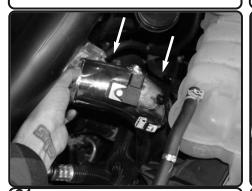
**21.** Install the new charge pipe. Secure the pipe and positon.
