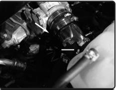
**22.** Install the 3-1/8"x 3-1/4step hump hose to the throttle body using provided clamps. Do not tighten.
