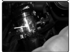
**23.** Secure the vacuum line and reconnect temperature sensor harness.
