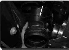
**12.** Pull back the plastic elbow from the intercooler.
