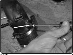
**19.** Loosen the torx screw holding in the temperature sensor. Remove the sensor.
