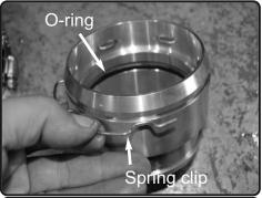
**16.** Install the o ring and the spring clip to the billet adaptor.
