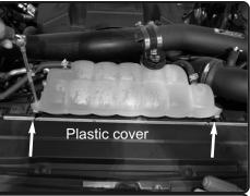
**2.** Loosen the 2 bolts holding in the coolant reservoir.
