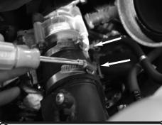
**6.** Loosen the clamp on the throttle body using 7mm nut driver.
