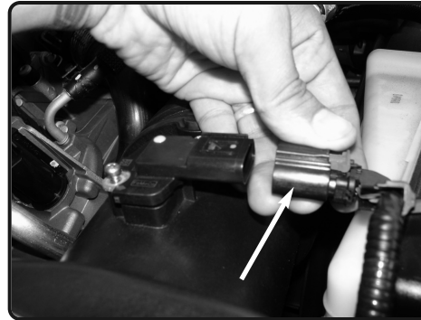
3. Disconnect the MAF sensor harness from the MAF sensor on the air box assembly.
