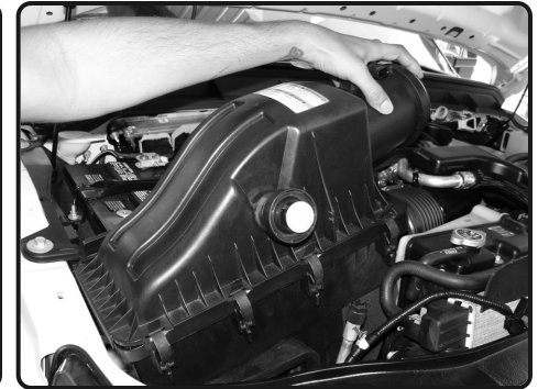
4. Lift the entire air box assembly out. Once air box is out. Remove the air duct from figure 3
