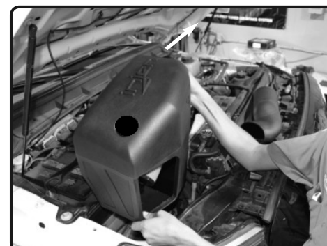
10. Drop the complete Injen airbox onto the mounting grommets from figure 10.
