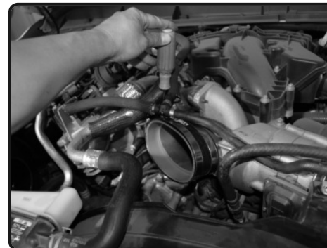
11. Place the 4.50" straight hose and two #72 clamps onto the turbo inlet. Only secure the clamp on the turbo inlet for now.
