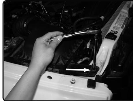
**3.** Remove the 10mm nut from the air box assembly on the radiator support.
