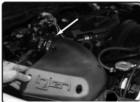
**13.** Place the 4.50" hump hose and two #72 clamps onto the intake plenum. Make sure you slide the hump hose as far back as you can.
