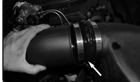
**17.** Push the upper part of the intake tube into the 4.50" hump hose on the intake plenum. Slide the hump hose towards the intake tube till it's centered. Adjust intake tube for best fitment and then secure all the clamps.
