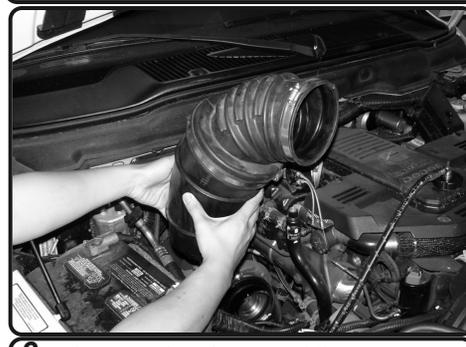
**6.** Loosen the clamp and the vacuum line on the air duct connected to the turbocharger inlet and crank case breather line and then remove the entire air duct.
