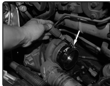
**15.** Place the 4.00" straight hose and two #64 clamps onto the turbo inlet and only secure the the clamp on the turbo side for now.
