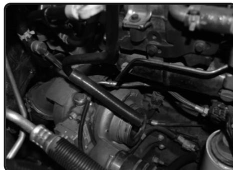
**14.** Connect the OE vacuum hose to the crank case breather line. This vacuum line will connect to the Injen intake tube in figure 17
