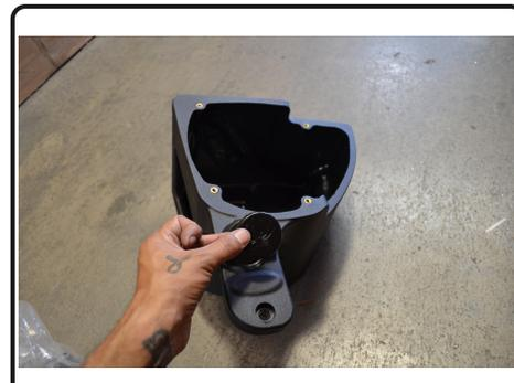
**10.** Place the supplied Filter Monitor Plug into the lower air box assembly.
