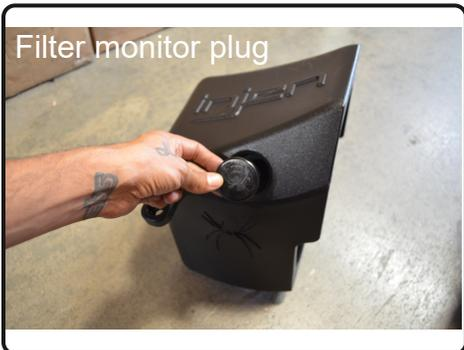
5. Place the Filter monitor plug into the drilled hole on top of the Injen air box.
