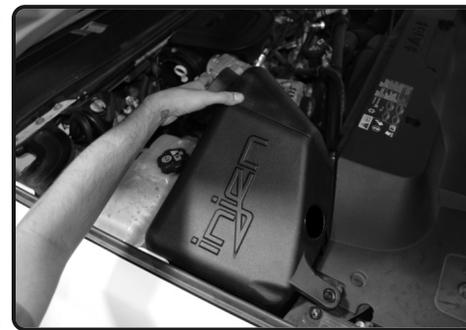
11. Lower the Injen air box into the engine bay. Make sure the pegs under the Injen air box goes into the factory air box grommets on the air box tray from figure 10
