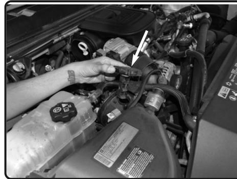
3. Remove the factory torx screws from the MAF sensor and then remove the MAF sensor from the factory air box assembly.
