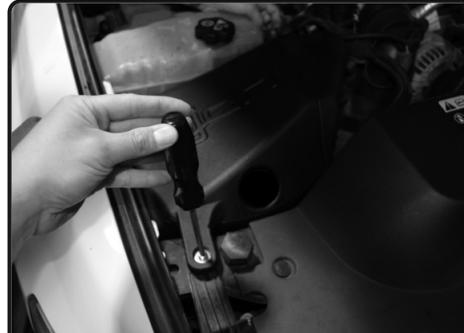
**16.** Reuse the factory 8mm bolt and secure the Injen air box bracket to the passenger side headlight bracket.
