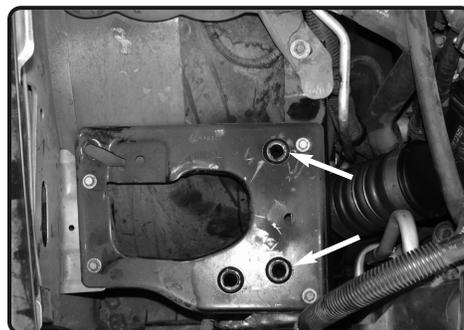
10. The factory air box assembly bracket is shown in the photo. Arrows indicate the grommets where the Injen air box mounts will go.
