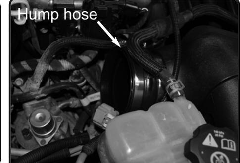
13. Place the 5.00" hump hose and two #80 clamps onto the Injen intake plenum on the injen air box.
