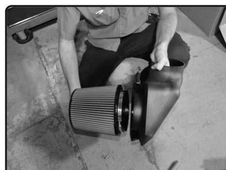
7. Place the filter onto the the Injen in-take plenum and then secure the clamp.
