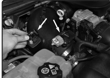
**15.** Place both MAF sensors onto their appropriate location and then screw them down with the supplied M4 bolts. Reconnect the MAF sensor harnesses
