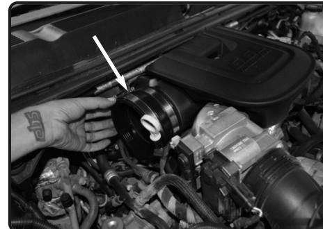
12. Place the 4.25"-4.50" step hose and two #72 clamps onto the turbo inlet. Tighten the clamp on the turbo inlet side for now.
