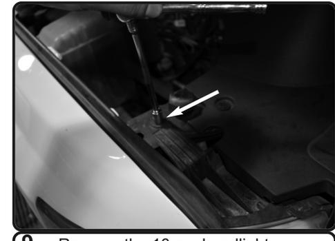
9. Remove the 10mm headlight bracket bolt on the passenger side head light. The Injen air box assembly will bolt up to this bolt.
