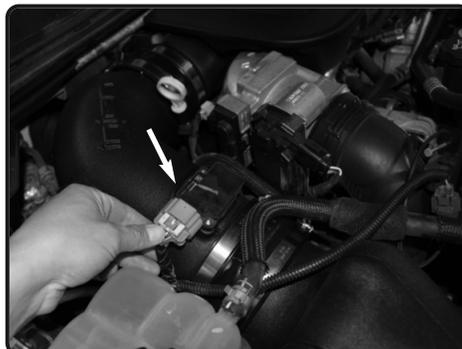
**15.** Place the MAF sensor onto the intake tube and then secure it with the supplied M4 bolts. Reconnect the MAF sensor harness.
