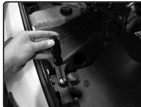
**16.** Reuse the factory 8mm bolt and secure the Injen air box bracket to the passenger side headlight bracket.
