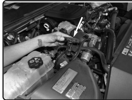
**3.** Remove the factory torx screws from the MAF sensor and then remove the MAF sensor from the factory air box assembly.
