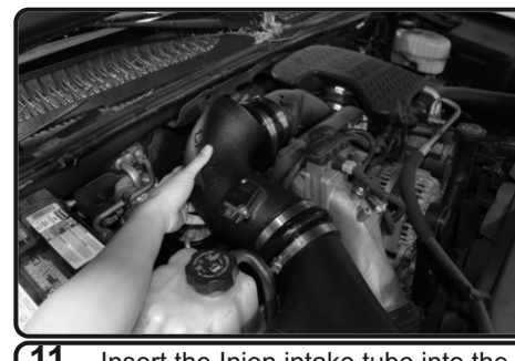
11. Insert the Injen intake tube into the 4.50" hump hose and the turbo end into the 4.25"-4.50" step hose. Once the intake is adjusted for best fitment, continue to secure the rest of the clamps
