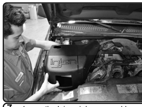
7. Lower the Injen air box assembly into the engine bay. Make sure the pegs under the injen air box goes into the factory air box grommets located on the air box bracket.
