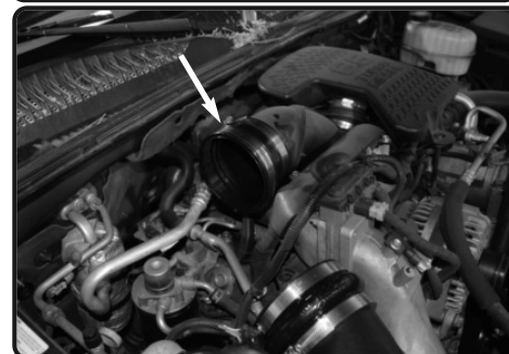
10. Place the 4.25"-4.50" step hose and one #72 and #64 clamps onto the turbo inlet. Tighten the clamp on the turbo inlet side for now.
