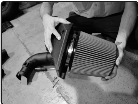
5. Place the filter onto the the Injen intake plenum and then secure the clamp.
