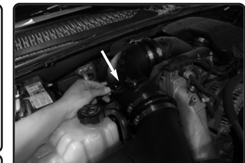
12. Re-connect the MAF sensor harness
