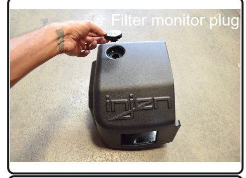
4. Place the Filter monitor plug into the drilled hole on top of the Injen air box.
