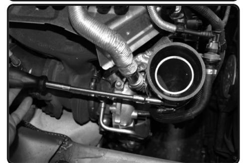
12. Tighten the clamp on turbo only.
