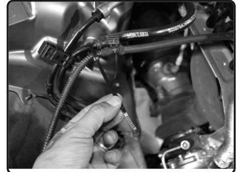
**20.** With provided zip ties, secure the MAF sensor and headlight harness. Re-install the plastic cover and secure.
