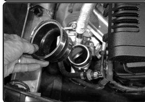
11. Install the provided step hose with clamps provided to turbo.
