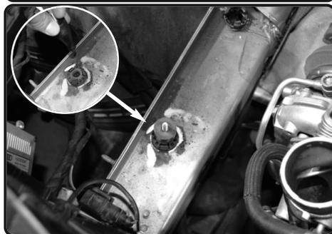
10. Now install the provided M6 stand off stud to the grommet that air box mounted to on frame. This will seat in the grommet.
