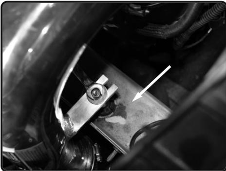
**17.** Once positioned, secure the bracket using provided M6 nut and fender washer. Secure and tighten using 10mm wrench or socket.
