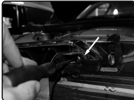
6. The other bolt will be located behind first bolt holding in plastic shroud. This will now have access to the remaining bolt.
