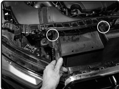
5. Locate the 2 bolts holding in the front air scoop and loosen and remove using T25 torx bit.
