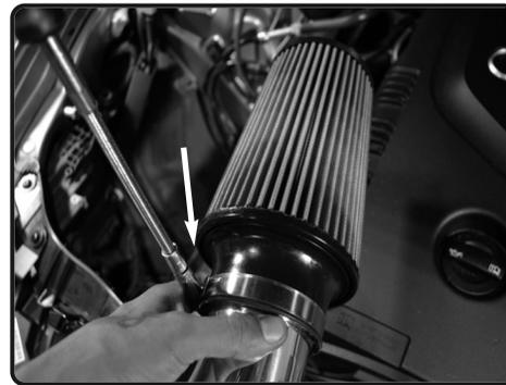
**15.** Install the filter to the intake tube and secure using 8mm nut driver.
