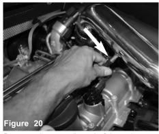
Re-connect the vacuum line to the fitting on the intake tube.
