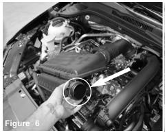
With pliers or channel locks, loosen the clamp on stock ram scoop. Pull back from the ram scoop. Lift up and remove the factory air box.
