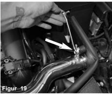
Secure and tighten the bracket using 10mm socket or wrench.
