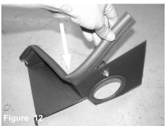
Install the rubber trim seal to the top of the heat shield. Notch corner with cutters or pliers for easier installation.
