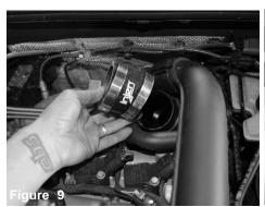
Install the 2.5" straight hose with clamps to the turbo housing. Tighten clamp on turbo only.
