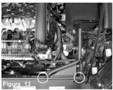
Now install the heat shield and position the tabs on heatshield to the factory ramscoop from step 7. Secure using factory screws.
