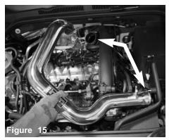
Install the intake into the vehicle and position the tube to hose on turbo and bracket to the vibramount on heat shield
