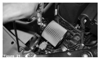
Install the air filter to the intake tube. Secure and tighten using 8mm nut driver.
