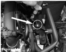
Tighten the rear tab using provided M6 allen screw and fender washer.
