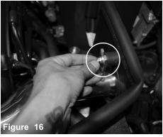
Secure the bracket on the heat shield using provided M6 nut and fender washer. Do not tighten.
