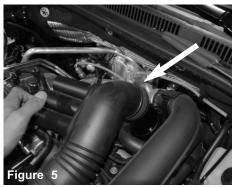
With pliers or channel locks, loosen the clamp on stock intake tube. Pull back the intake tube from the turbo housing.
