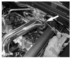
Tighten the clamp on turbo side using 8mm nut driver
