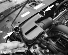
Loosen the 2 screws holding in the ram scoop using T25 torx bit or screwdriver. Save the screws for later install.
