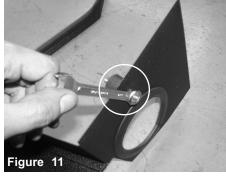
Install the vibramount to the heat shield and secure using provided M6 nut.
