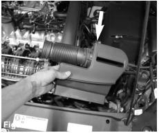
Pull back the ram scoop out of the vehicle.
