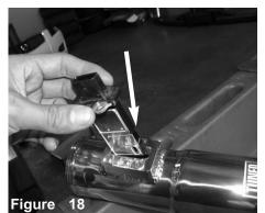
Install the MAF sensor into the intake tube.
