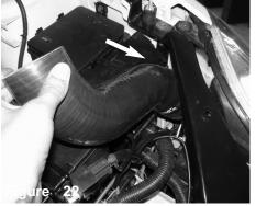
Now install the molded silicone hose behind the headlight. Install the injen logo side first down.
