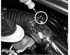
Position for best fit and tighten using 8mm nut driver.
