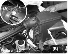
Loosen the clamp on the air box using 8mm nut driver(A) The air box cleaner is now ready to be pulled out from the engine compartment(B)
