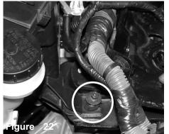
Now that the tray has been lifted out of the way, continue to loosen the m6 bolt located on the corner of the air box.
