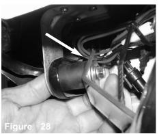
Secure the bracket using provided M6 nut and washer. DO NOT TIGHTEN<
