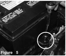
Loosen the m8 bolt located on the tray bracket, once the bolt has been loosened, this will allow the base of the battery to un-wedge itself from the tray.
