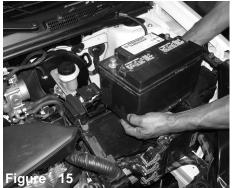
Place the plastic battery tray over the metal battery holder and set the battery back to its original location. Re-secure the battery and continue the install.
