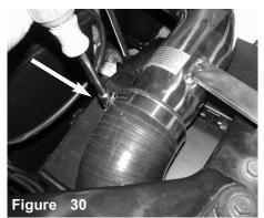
Position for best fit and tighten clamp using 8mm nut driver.
