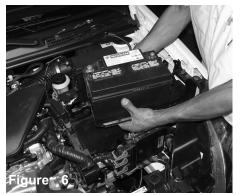
Remove the battery cables and carefully pull the battery out of the engine compartment for now.
