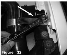
Secure the bracket and tighten using 12mm socket and or wrench.
