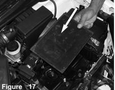
Remove the plastic battery tray from the metal battery holder, this will give you access to the five bolts under the plastic tray.
