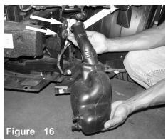
Remove the resonator from the vehicle.
