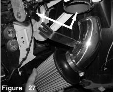
Install the filter to the lower intake assembly tube. Now position bracket to the vibra mount and silicone hose. DO NOT TIGHTEN<
