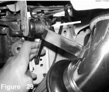
Now position for the best fit, check clearance with the whole intake system and tigthen the bracket using 10mm wrench. Tighten clamp using 8mm nut driver.
