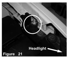
Locate near fender where there are 2 bolts. Loosen the 2nd bolt, using 13mm socket and extention, closes to the firewall. Remove and secure with provided M8 vibra mount.
