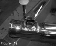
Now secure the MAF sensor using the factory screws and tighten using 7mm nut driver.
