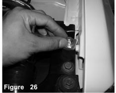
Secure the bracket using M8 nut and washer. DO NOT TIGHTEN<
