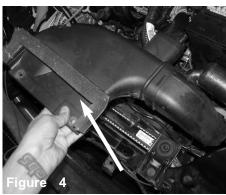
Remove the 2 push clips that hold in the factory snorkel unit and remove.
