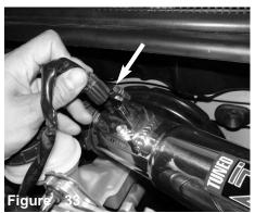
Re-connect the MAF sensor harness. Re-connect the battery and re-install the bumper cover.
