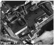
Once all four bolts have been removed, lift and tilt the tray over to one side to allow access to the last m6 bolt.
