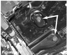
Bolts (C) and (D) are removed next. This will now give you access to the last m6 bolt securing the air box cleaner.
