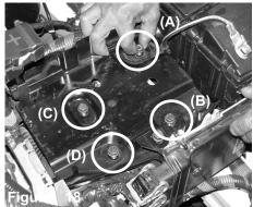
Loosen and remove all four m8 bolts from the battery tray as shown above. Start by removing bolt (A) from the metal battery tray.
