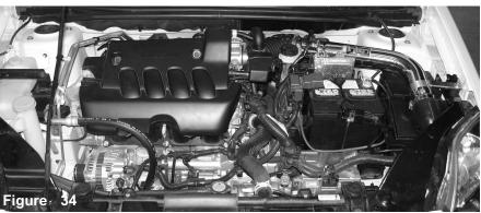
Congratulations! You have just completed the installation of this intake system. Periodically, check the alignment of the intake, normal wear and tear can cause nuts and bolts to come loose. <u>Note: Check</u> clearance and adjust if needed! Failure to check the alignment and adjust the intake can cause damage that will void the warranty. Injen Technology is not responsible for any damages caused by/from improper installation.
