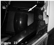
Position like image above. Make sure any wires are not in the way of the silicone hose.
