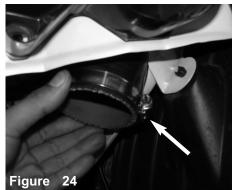
Now when positioned like above attach the clamp to the silicone hose.
