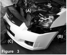
Remove all four clips on top bumper (A), two m6 bolts under the fender well(B), six phillips screws and five clips located under the bumper (C). Now carefully pull the bumper away from the frame.
