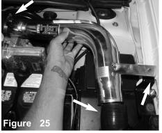
Install the upper intake tube and position the bracket to the vibra mount, and to the stock hose connected to the throttle body and silicone hose. DO NOT TIGHTEN<
