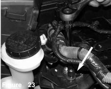
The m6 bolt located over the extended leg on the air box cleaner is now being removed.
