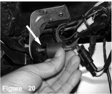
Locate the M6 thredded stud under the headlight. Now secure the female side to the vibra mount and tighten.
