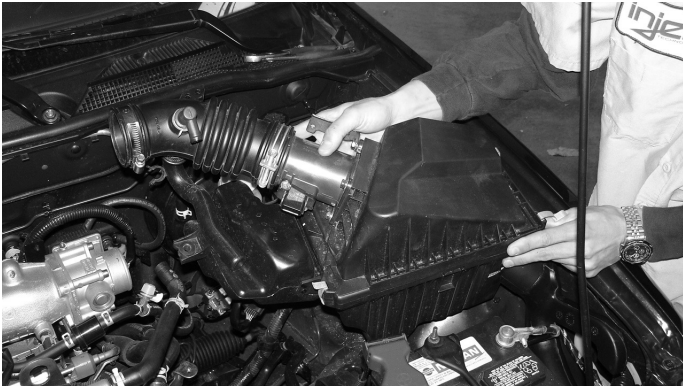
Loosen the clamp on the throttle body, remove the crankcase breather hose and remove the entire air intake box and air intake duct.
