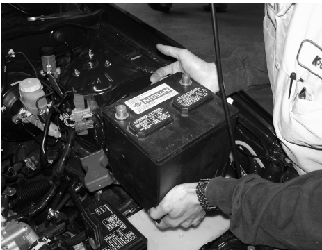
Disconnect the battery terminals from the battery, loosen the battery tie down and continue to remove the battery from the engine compartment.
