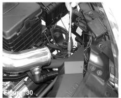
With adjustable torx snake, tighten both screws.
