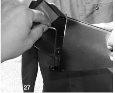
With screw, install and hold with torx key.
