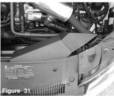
Make sure the power-ram is secure and tighten.
