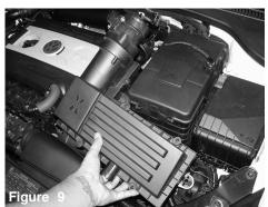
Pull out the complete air box assembly.
