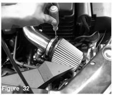
Install the filter and secure using 8mm nut driver.
