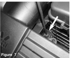
With T30 torx bit, loosen the screw holding in air box.
