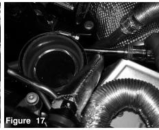
Tighten the clamp on the turbo only using 8mm nut driver.
