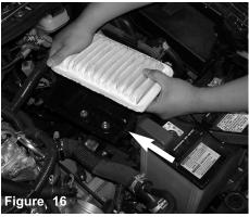
The stock filter panel is removed from the lower air
