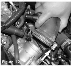
The air duct clamp is loosened at the throttle body, once the clamp has been loosened the air duct is ready to be pulled off.
