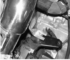
The primary intake bracket is aligned to the upper vibra-mount stud.
