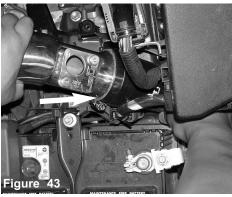
The silicone hose is pressed over the primary intake, use one power band to fastened the silicone hose over the intake end.
