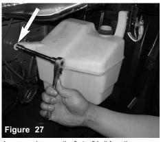
Loosen and remove the first m6 bolt from the reservoir bottle as shown above.
