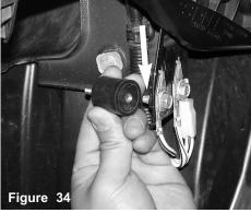
Close up of the male/female vibra-mount aligned to the bolt. The bolt is located behind the reservoir bottle.
