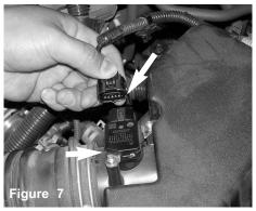
Depress the tab and pull the electrical harness connector from the mass air flow sensor.
