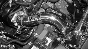
Periodically, check the fitment of both intake systems. Normal driving conditions may loosen nuts, bolts and clamps causing intakes to shift resulting in damage to automotive parts.
