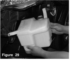
The reservoir bottle is temporarily removed in order to install the cold air intake.
