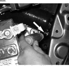
The silicone hose clamp is now tightened as shown above.
