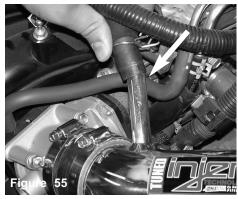
The crankcase hose is now pressed over the intake vacuum port.
