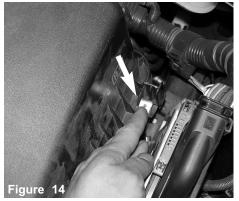
The second metal clamp is unhooked from the upper air box.
