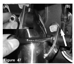
The m6 nut and washer are placed over the intake bracket (A), continue to tighten the m6 nut as shown above (B).
