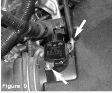
The stock screws are loosened and removed from the mass air flow sensor
