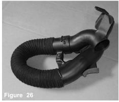
The air resonator hose will no longer be used with the cold air intake.
