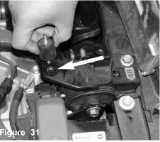
The male vibra-mount is aligned and fastened to the motor mount bushing.
