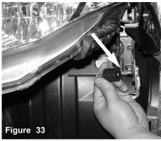
The male/female vibra-mount is aligned to the exposed bolt that holds down the grounding wires.
