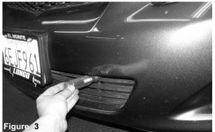
Prior to starting the installation, remove the 2 plastic clips inside of the grill.
