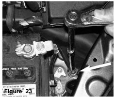
A ratchet and 10mm socket is used to loosen the bolt.
