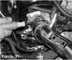
Once you have aligned the intake system, you may now tighten the clamp.
