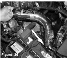
The primary intake is lowered into the engine compartment and into the front bumper.
