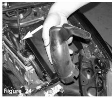
The resonator air scoop is now ready to be removed.
