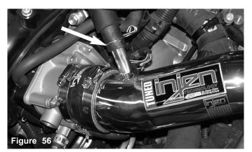
The crankcase hose is pressed over the intake port and the tension clamp is placed over the intake vacuum port.
