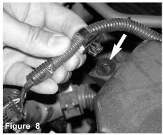
The harness clip is pulled out from the air box attachment as shown above.
