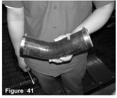
The 55 degree silicone hose and clamps are assembled as shown above.
