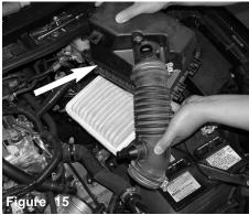
The upper air box is detached from the lower air box and air intake duct is removed from the throttle body.
