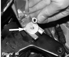
The m6 flange nut and washer is used to fasten the intake bracket to the vibra-mount stud.
