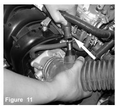
The crank case hose is removed from the air duct vacuum port.
