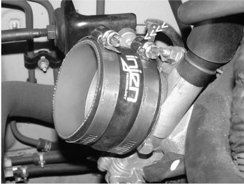
Press the 2 3/4" straight hose over the throttle body. Use two power-bands on the hose and tighten the band on the throttle body side for now.
