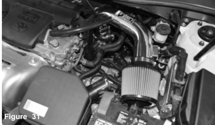
Figure 31 Congratulations! You have just completed the installation of this intake system. Periodically, check the alignment of the intake, normal wear and tear can cause nuts and bolts to come loose. Failure to check the alignment and adjust the intake can cause damage that will void the warranty.
