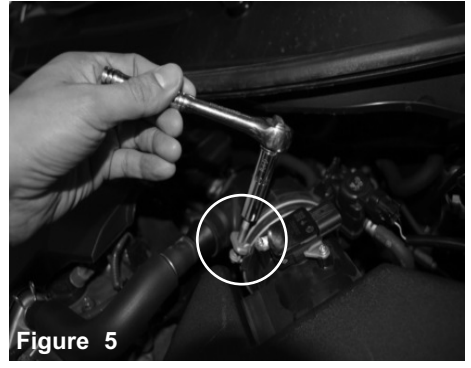
Figure 5 Loosen the clamp on the air box using 10mm socket or wrench.
