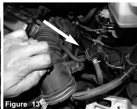
Figure 13 Pull apart. With clamps, de-press the clamp on the throttle body.
