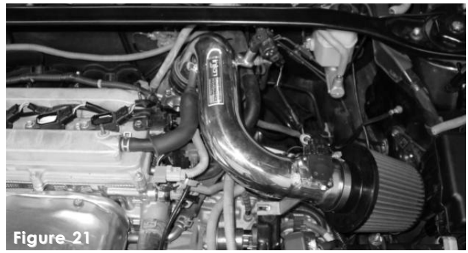
Figure 21 Start your engine and listen to any possible air leaks, rattles or rubbing. If you come across any problems, go back and recheck any connections and retighten all nuts, bolts and clamps. Periodically, check the fitment of the intake system for any possible movement, this will prevent any possible damage to the intake.
