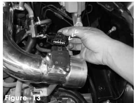
Figure 13 Press the electrical harness clip into the mass air flow sensor.
