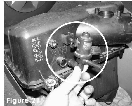
Figure 18 The breather hose is now attached to the intake port.
