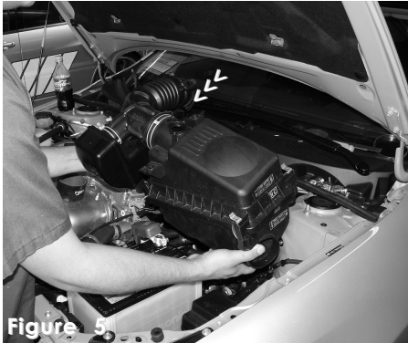
Figure 5 Loosen the clamp on the throttle body, now pull the entire air box cleaner out of the engine compartment.
