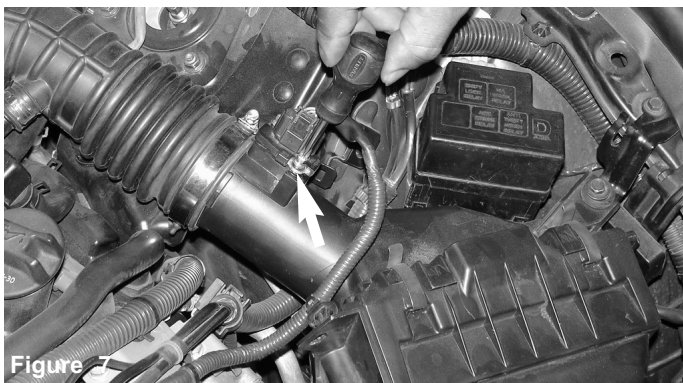
Figure 5 The stock m6 bolt has been removed for now.
