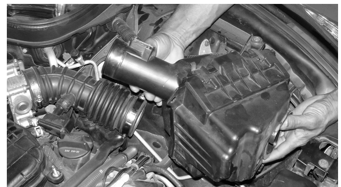
Figure 8 Once you have removed the sensor bolts, continue to pull the mass air flow sensor from the sensor housing.
