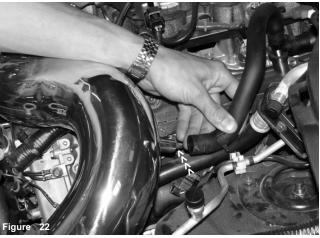
Press the stock breather hose over the end of the large intake port, use the stock clamp to secure the hose to the intake port.
