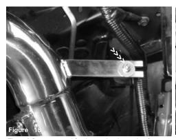
The m6 flange nut and fender washer is used to fasten the intake bracket to the vibra-mount stud.
