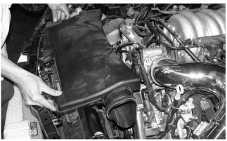
Replace the front air scoop back to its original position once the intake has been installed.
