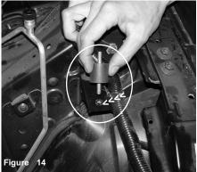
The vibra-mount is screwed into the fender well air box bracket as shown above.
