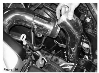
Lower the secondary intake into the large resonator opening while carefully aligning the intake bracket to the vibra-mount stud.
