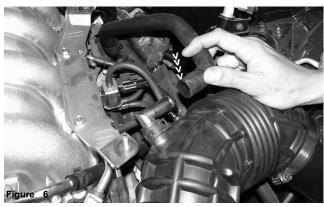
Use pliers to press the tension clamp on the breather hose. Pull the tension clamp back and remove the breather hose from the air intake duct.
