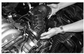
Loosen clamps on both ends of the air intake duct. Once clamps have been loosened, continue to pull the air duct from the throttle body and air box cleaner.
