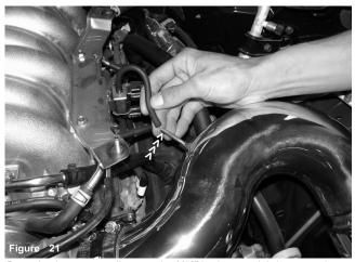
Press the 4mm vacuum line over the 3/16" intake port. It is important that the Vacuum switching valve hose be securely placed over the 3/16" intake port. A bad connection will cause idling problems if not installed properly.
