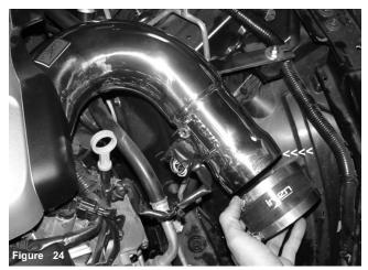
The power -bands are placed over the 3 1/2" straight hose. Press the straight hose over the end of the primary intake, approximately one inch of the hose is pressed over the intake end.
