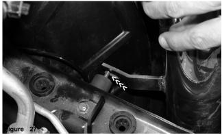
align and set the intake bracket over the vibra-mount stud. Press the top end of the secondary intake into the hose located on the primary intake.
