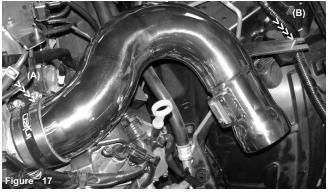
The intake is pressed into the throttle body hose (A) while the intake bracket is aligned to the vibra-mount stud (B).
