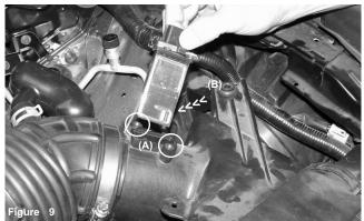
Remove the two screws from the sensor housing (A) pull the mass air flow
