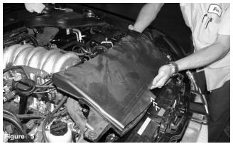
Remove plastic clips from the front air scoop and remove the entire air scoop from the top cross member.
