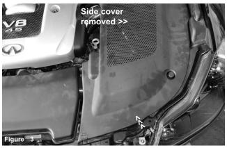
The plastic clips used to secure the side cover are removed and the entire plastic side cover is removed from the engine compartment.
