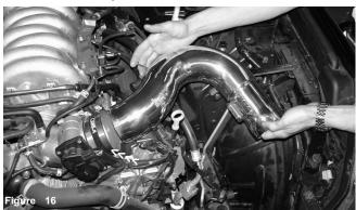
The primary intake is lowered into the engine compartment while the top end is pressed into the throttle body hose.
