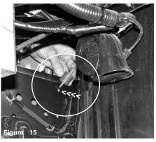
The second vibra-mount is screwed into the pretapped hole located on the main frame.
