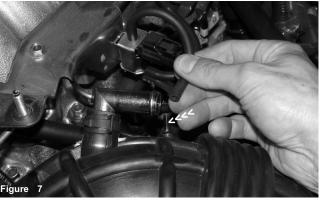
Pull the 4mm vacuum hose from the stock air intake duct as shown above.
