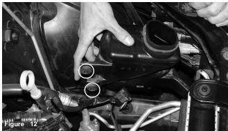
Pull the resonator box out of the grommet pins used by the resonator box. The resonator box will not be used as part of this installation.
