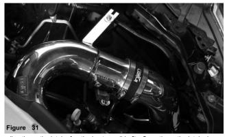
align the entire intake for the best possible fit. Once the entire intake has been checked and cleared for any possible rubbing or rattling, continue to tighten all nuts, bolts and clamps.
