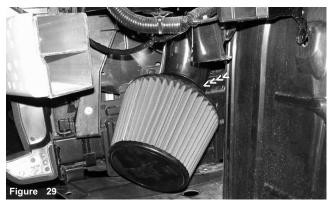
Press the filter over the end of the secondary intake. Once the intake has been butted to the filter stops, continue to tighten the filter neck clamp.
