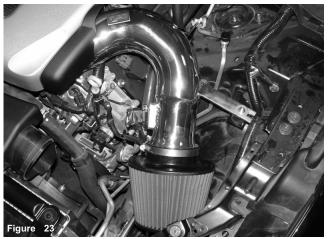
The SP1996 cold air intake can also be used as a short ram. It is recommended to use the system as a short ram whenever rain is expected.
