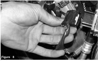
Remove the electrical clip from the mass air flow sensor located on the sensor housing.
