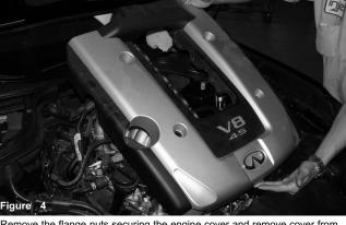
Remove the flange nuts securing the engine cover and remove cover from the engine compartment.
