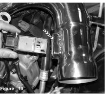
Insert the mass air flow sensor into the machined adapter. Once the mass air flow sensor has been butted up to the adapter, continue to use the stock screws to fasten the sensor and adapter together.
