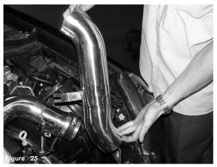
The secondary intake is lowered into the engine compartment.
