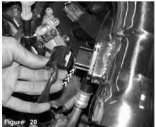
Press the electrical harness clip over the mass air flow sensor. A firm snap is a sign of a good connection of the two devices.
