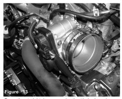
Press the straight hose over the throttle body and use two power bands. Once the hose has been placed over the throttle body, use a nut driver to tighten the power band on the throttle body side.
