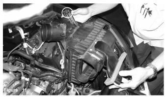
Remove screws used to hold the air box cleaner in place. Once screws have been removed, continue to pull the entire air box cleaner out of the engine compartment.
