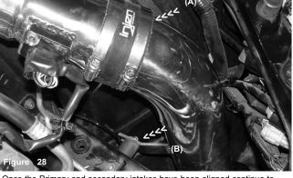
Once the Primary and secondary intakes have been aligned continue to semi-tighten the power-band (A). Use the m6 flange nut and fender washer to secure the intake to the vibra-mount stud (B).
