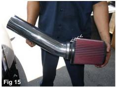
Take the secondary intake and press the large Injen filter over the end of the intake. Once the filter has been positioned in place, fasten clamp located on the filter neck.
