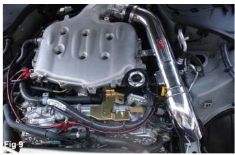
Align the entire intake for best possible fit then continue to semi-tighten nuts, bolts and clamps just enough to hold the intake in place.
