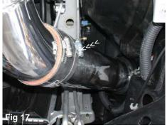
Insert the top end of the secondary intake into the 3 1/2" straight hose located over the primary intake. Semi-tighten the .412 power-band to hold both intakes together.
