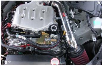
Short ram installation- Press the Injen filter over the end of the intake and fasten clamp located on the filter neck. Align intake for best possible fit. Once fitment has been cleared continue to tighten all nuts, bolts and clamps.
