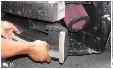
Once a corner section has been cut off, place it in back in the stock location. Cut just enough to give you about 1/4" to 3/8" clearance between the filter and foam insolation. Direct air to the filter will cause air turbulence that will cause the engine to stall. Do not remove foam insulator from car, must be used.
