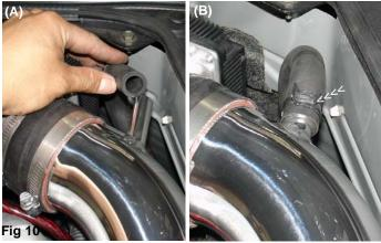
Find the stock breather hose and press it directly over the 1/2" intake port (A). Once the breather hose has been pressed over the intake port, use the stock clamp to prevent the hose from slipping off (B).
