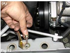
Remove the m6 stock bolt securing the air conditioning bracket to the frame.
