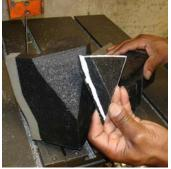
Take the foam insulator located in the front bumper and use a bandsaw, hack saw or saw that is capable of slicing through foam. It will be necessary to cut a corner piece from the foam insulator in order to make room for the filter. Start by cutting about an 1" as shown in figure (A) and (B). Do not remove foam from the bumper support.
