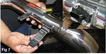
Locate the primary intake and carefully insert the air mass sensor into the machined flange welded to the intake (A). Use the stock screws to fasten the sensor in place (B).
