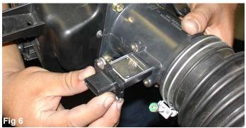
Using the torx bit in this kit, remove the screws holding the mass air sensor to the sensor housing. Gently, proceed to remove the sensor from the sensor housing as shown in this picture.
