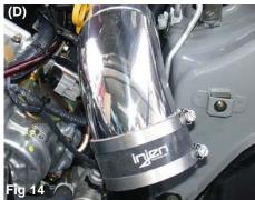
CONTINUING TO INSTALL SECONDARY INTAKE-Press the 3 1/2" straight hose over the end of the primary intake. Use two large clamps and only tighten the clamp located on the end of the intake (D).
