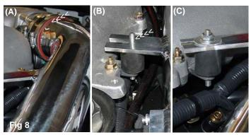
Press the intake outlet into the throttle body hose (A). Align the intake bracket to the vibra-mount stud (B). Place the fender washer over the stud and screw the m6 flange nut on the stud (C).
