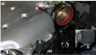
Press the 3 1/8" straight hose over the throttle body and use two .362 power-bands on the hose. Tighten the band on the throttle body side in order to prevent the hose from slipping off (A). Take the vibra-mount and screw it into the pretapped wing located to the side of the intake manifold cover (B). Vibra-mount fully installed (C).
