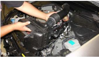
Loosen all clamps and remove bolts that holds the air intake duct and air intake box in place. Gently, remove the entire air box assembly from the engine compartment and set it aside.
