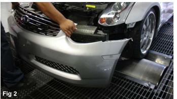
This installation will require the removal of the front bumper. Refer to page three for step by step instructions. Loosen clamps at the throttle body and the air box. Un-clip all hinges on the air box lid. Remove the air box lid and the stock air filter, then continue to remove the lower air box cleaner.
