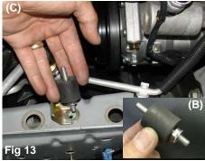
Find the remaining vibra-mount and screw an m6 nut as shown in picture (B) With the m6 nut facing down, screw the vibra-mount into the bracket and frame (C).
