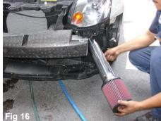
Insert the top end of intake into the driver side bumper and up through the engine compartment.
