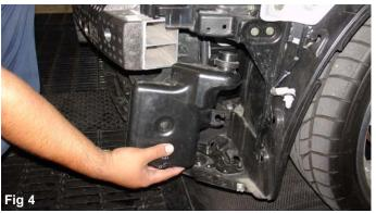
Once the bumper has been removed continue to unscrew the m6 bolt then remove the air resonator box from the driver side bumper. The removal of the resonator box will allow room for the air filter and secondary intake assembly.
