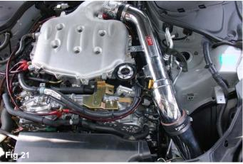
Congratulations! You have just completed the installation. Periodically, check the fitment of the intake system to make sure no rubbing is damaging the intake. Failure to check the intake will cause permanent damage to the intake system.
