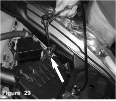
A 10mm socket is used to loosen and remove the 10mm bolt holding the air box cleaner in place.
