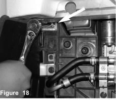
The second 10mm bolt is removed from the front of the reservoir bottle.
