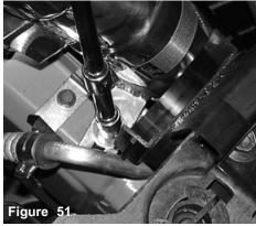
using a 10mm socket and 3/8 rachet, tighten the 10mm bolt securing the pipe to the stand-off.
