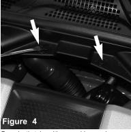
Pop plastic tabs with screwdriver and remove clips from the stabilizer bar upper cover.
