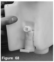
Pump secured to the Injen reservoir bottle.
