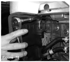
use a 10mm socket and 3/8 rachet to tighen the 10mm bolt to secure the side bracket to the radiator support
