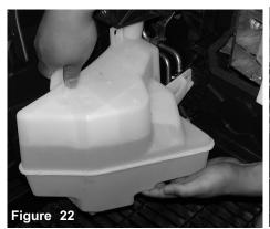
The reservoir bottle fluid is poured into a container to be useded later in the instruction.
