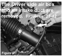
The electrical harness is disconntec from the mass air flow sensor.
