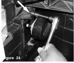
The 10mm bolt holding the horn in place is loosened.
