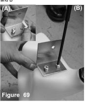
Place the upper reservoir bottle bracket over the two nut inserts on top of the Injen reservoir bottle and secure it with twoM6 hex bolts.
