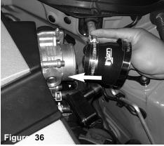
Press the silicone step-hose over the throttle body until it sits flush up against the base of the throttle body.
