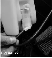
Place water line back into the water pump
