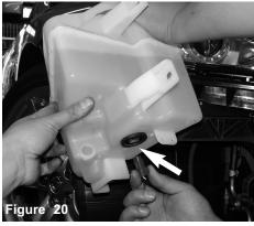
The electrical harness clip is removed from the reservoir sensor as shown above.
