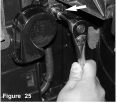
Once you have loosened the 10mm bolt, continue to turn the horn downward, re-tighten the 10mm bolt.
