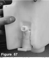
Place stock pump into the grommet that was place into the Injen reservoir bottle. A litlle WD40 on the grommet might help with inserting the pump.
