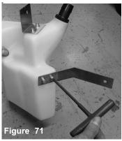
Tighten the two M6 hex bolts to secure bracket onto reservoir bottle.
