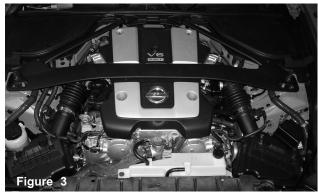
Stock air intake cleaner and air ducts shown in this picture. Before getting started with the installation, disconnect the negative battery terminal.
