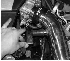
Insert the CCV breather box into the 15mm vacuum hose.
