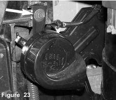
The driver side horn bolt is loosened in order to reposition the horn.
