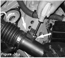
The two screws holding the mass air flow sensor to the sensor housing are removed.
