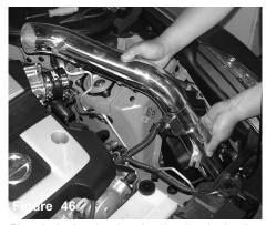
Place the intake tube down into the the wheel well.
