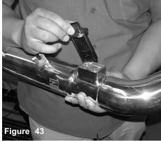
Carefully insert the mass air flow sensor into the sensor housing of the intake pipe.
