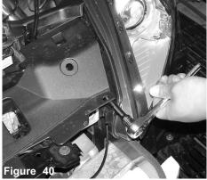
Remove the 10mm bolt securing the factory air box duct from the front side of the radiator support.
