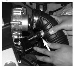
Pull the air duct from the the throttle body and pull the intake port from the CCv box.
