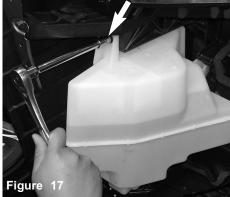
Thr first 10mm bolt is removed from the reservoir bottle frame.
