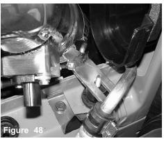
Align the intake bracket over the stand-off.
