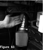
Make sure the end of the 25mm hose drops through the bottom near the filter on the passenger side.
