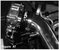
Place the throttle body end of the pipe into the silicone step-hose.
