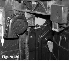
The horn is relocated so that the opening is pointing downward.
