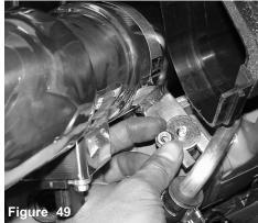
Place a fender washer and one M6 flanged nut onto the stud of the stand-off
