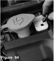
Filler spout in it's original location and use original plastic clipt to secure it.
