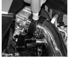
Once the pipe is aligned and there is clearance along the pipe, you may now tighen the clamp securing the
