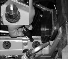
Align the composite stand-off over the front stock air box grommet and make sure it is fully inserted
