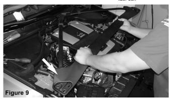
Once you have removed all nuts and bolts, continue to pull the stabilizer bar out of the engine compartment.
