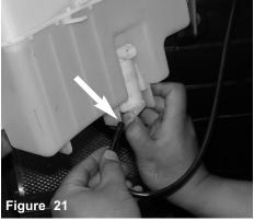
The motor vacuum hose is removed from the s reservoir motor
