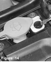
In order to remove the spout, the plastic tab is popped and removed
