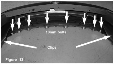
Remove all 8- 10mm bolts located under the bumper and two side clips
