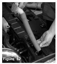
Insert the 25mm hose into the original locaation of the spout.
