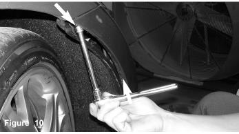
Remove the 10mm bolt located on the passenger and driver side upper wheel well.
