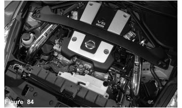
.Congratulations! You have just completed the installation of one of the best air intake systems on the market. Prior to driving, start the engine and listen for odd sounds such as rattling, rubbing or vacuum leaks. If everything checks out fine, let it idle for 10 minutes in order for the ECU adjust to the added volume of air.
