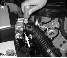
Loosen the air intake duct clamp located over the throttle body.
