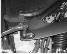
Passenger side strut tower- Loosen and remove two 14mm bolts and one 14mm flange nut from the stabilizer bar.
