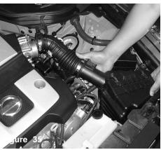
Continue to pull the entire air intake box cleaner and air intake duct from the engine compartment.
