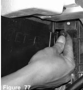
use a stock 10mm bolt and secure the side reservoir bracket to the stock location of the upper side bracket only.
