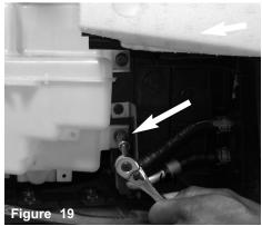
The third 10mm bolt is removed from the front of the lower reservoir bottle.
