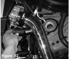
Place one 2"-15mm vacuum hose over the nipple located on the pipe
