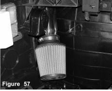
Use a 8mm nut driver to secure the filter to the end of the intake pipe.
