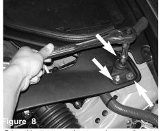
Driver side strut tower- Loosen and remove the 14mm bolts and one 14mm flange nut.
