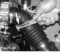
Compress the tension clamp on the CCV box and slip back. This will allow you to remove the CCV box.
