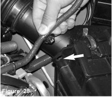
The harness tab is pulled off and removed from the corner air box.
