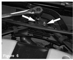
The stabilizer bar upper 14mm bolts are loosened and removed
