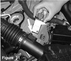
Once you have removed the two screws, continue to pull the mass air flow sensor from the sensor housing.
