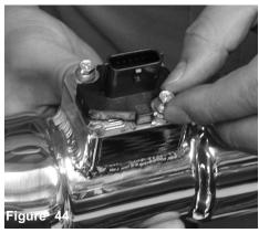
Re-use the stock M4 bolts to secure the air mass sensor to the sensor housing
