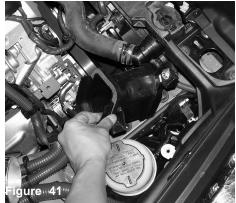
From the back side of the radiator support, remove the air duct
