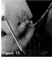
Insert harness back into the pump and make sure it snaps into place.
