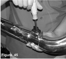
Use a 7mm nut driver to tighen the M4 bolts to the sensor housing.
