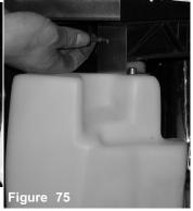
Using a stock 10mm bolt secure the upper reservoir bracket in it's stock location.
