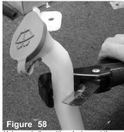
Using a similar cutting device, cut the reservoir spout at the beginning of the second bend.
