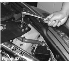
Continue to tighten all 14mm bolts securing the stabilizer bar. Remember to re-install the plastic cover for the stabilizer bar removed in figure (4)
