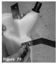
Place the lower reservoir bracket over the two nut inserts on the side of the reservoir bottle and insert two M6 hex bolts to hold it in place
