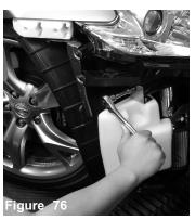
Tighten the 10mm bolt with a 10mm socket and 3/8 rachet.
