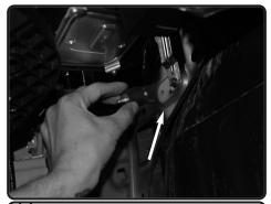
**14.** Locate the thredded insert from OEM resonator tube, install provided M6 vibramount.
