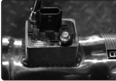
11. Now install the MAF sensor into the intake tube. Secure and tighten using OEM screws from previous step.
