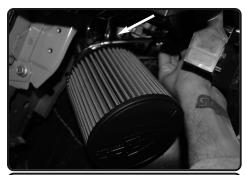
**24.** Install the filter to the lower intake assembly and tighten the clamp using 8mm nut driver.
