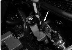
**21.** Secure the filter and tighten clamp using 8mm nut driver.
