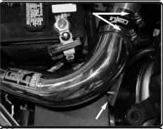
**19.** Connect the 2 pipes together. Tighten the clamps on the straight hose. Secure the brackets using fender washers and nuts.
