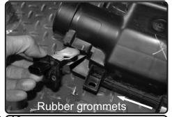
**10.** Loosen and remove the 2 screws holding in the MAF sensor using 7mm nut driver. Save screws for later install. Remove the MAF sensor.
