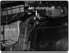
**15.** Secure the heatshied using provided fender washers and M6 nuts. Bracket in back corner will only have nut, no fender washer.
