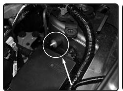
**12.** Install the provided female/male M6 vibramount to the thredded stud on strut tower, secure and tighten.
