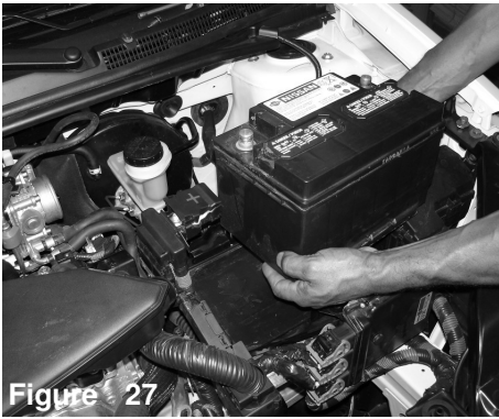
Figure 27 Place the plastic battery tray over the metal battery holder and set the battery back to its original location.
