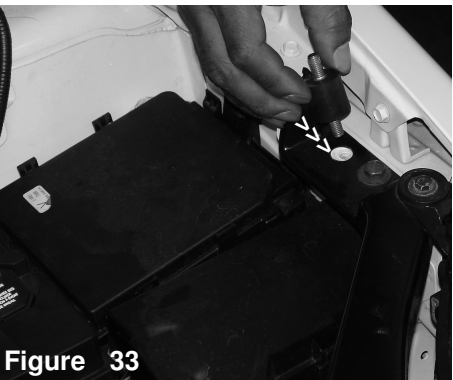
Figure 33 Align and screw the m8 vibra-mount into the fender well bracket as shown above.
