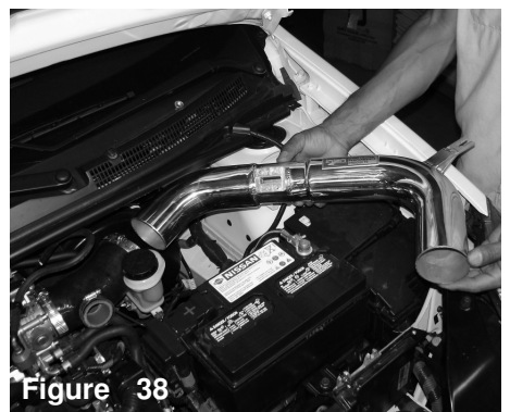
Figure 38 Align the intake to the formed silicone hose. Press the intake into the silicone holes while aligning the intake bracket to the vibra-mount stud.
