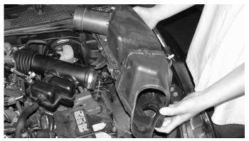
Loosen and clamps and bolts and remove the stock air intake box as shown above.
