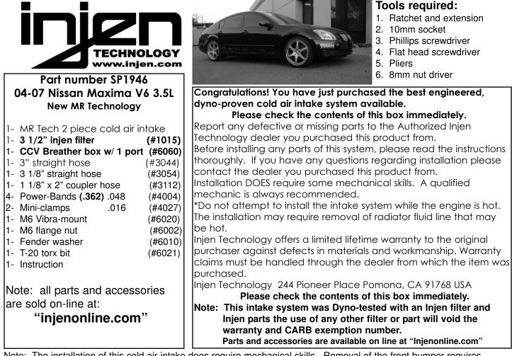
Note: The installation of this cold air intake does require mechanical skills. Removal of the front bumper requires loosening and removing several plastic plugs and screws that may be difficult. It is recommended that this system be installed by a professional mechanic. Be sure to disconnect the negative terminal before proceeding. Congratulations! You have just purchased the worlds first tuned intake system. MR Technology, Leading the way!
