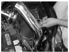
Carefully, lower the secondary intake into the resonator opening and into the bumper corner.
