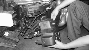
Once the bumper has been removed continue to disconnect and remove the plastic air intake resonator box.
