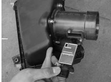
Use the torx bit in this kit to unbolt screws from the MAF sensor. Carefully, remove the MAF sensor from MAF sensor housing.
