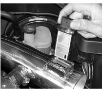
Take the MAF sensor and insert it into the machined MAF sensor adapter.
