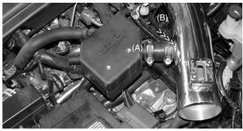
Press the assembled CCV box over the large intake port as shown above (A). Adjust entire CCV box and tighten clamp on the intake port (B).
