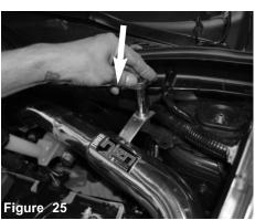
Adjust the intake system, tighten the bracket using 10mm socket or wrench.
