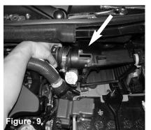
Detach the air duct hose from the air box housing.
