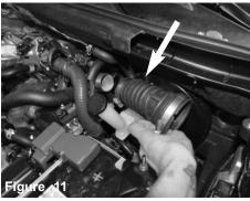
With 8mm nut driver, loosen the clamp on the turbo. Remove the stock turbo auxillary hose.
