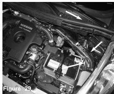
Position for the best possible fit. Make sure nothing is hitting or rubbing indicated by the arrows. Loosen the clamp and the vibra mounts and adjust if necessary for better fit.
